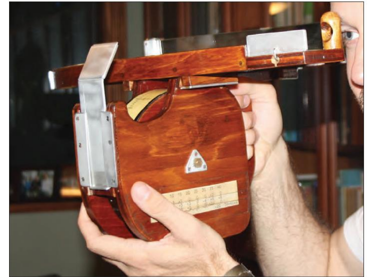
Walter Bitterlich's prototype relascope. Photo by Kim Iles.
