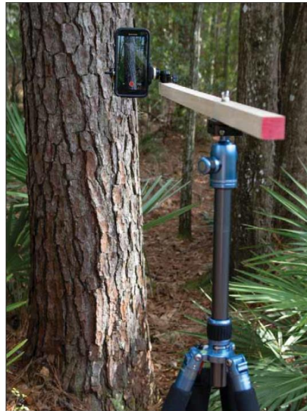
This simple wooden arm, mounted on a camera tripod, lets the author collect high-quality imagery that's later processed by the Google Cardboard app into three-dimensional imagery. Photo: Charlie Houder.
