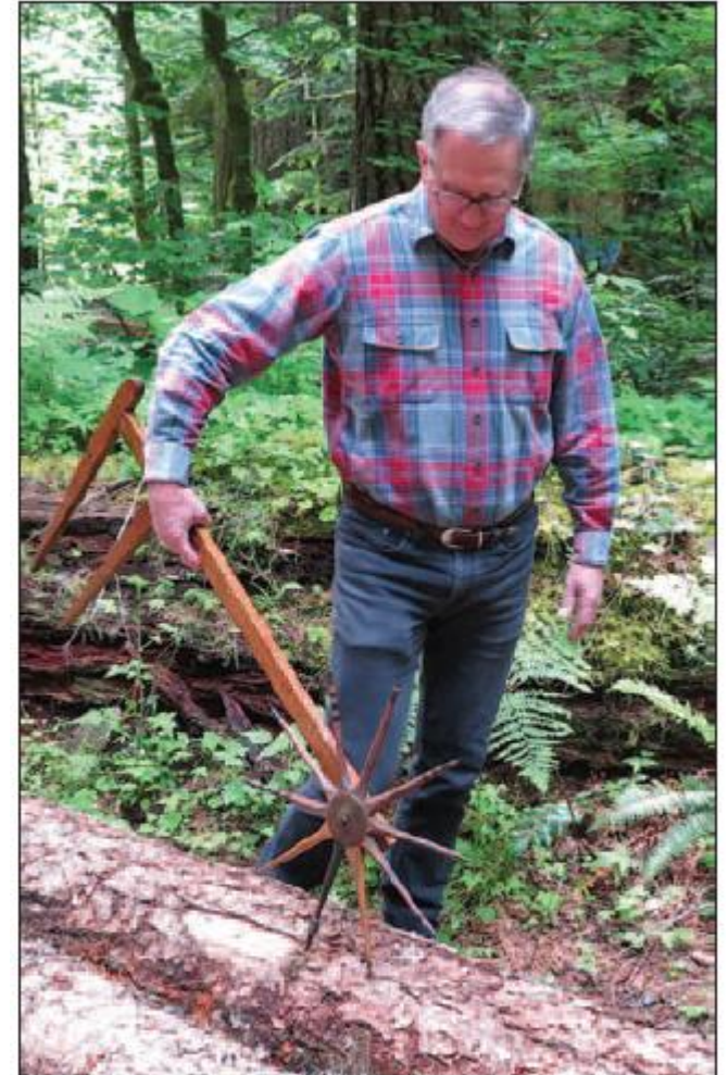
Steve Fairweather demonstrates his wheeled calipers, a model made in Maine by C.W. Grover, probably in the late 1800s or early 1900s. Photos by Steve Wilent.
