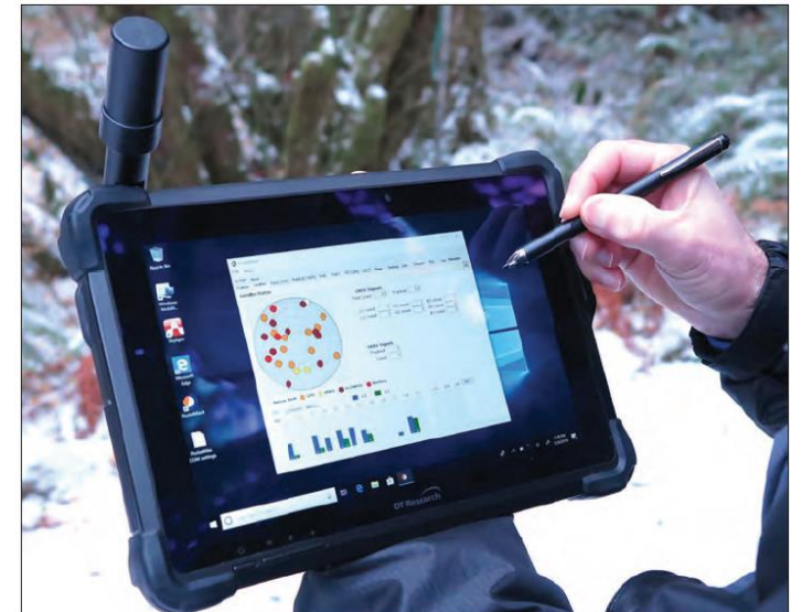
Figure 1. DT Research's DT301T Rugged RTK Tablet with the detachable Harxon GNSS antenna. Photo by Steve Wilent.
